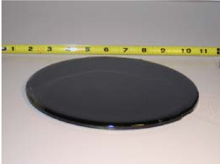
Fig. 3.17: An ultra-smooth 20 cm diameter flat mirror.
