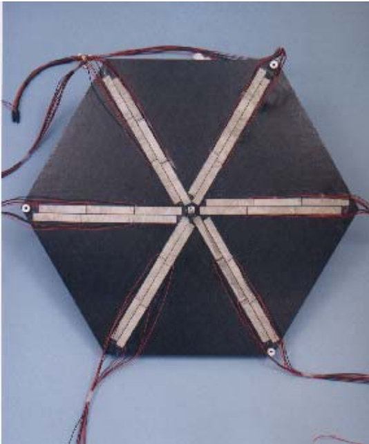
Fig. 3.18. The SI can use a simple proven scheme to adjust shape, focal length, and correct for thermal gradients.
