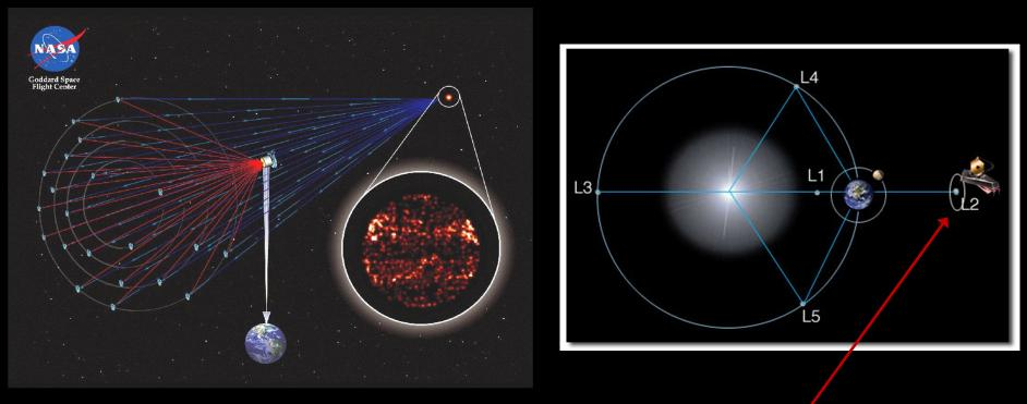
A 0.5 km diameter UV-optical Interferometer near Sun-earth L2
