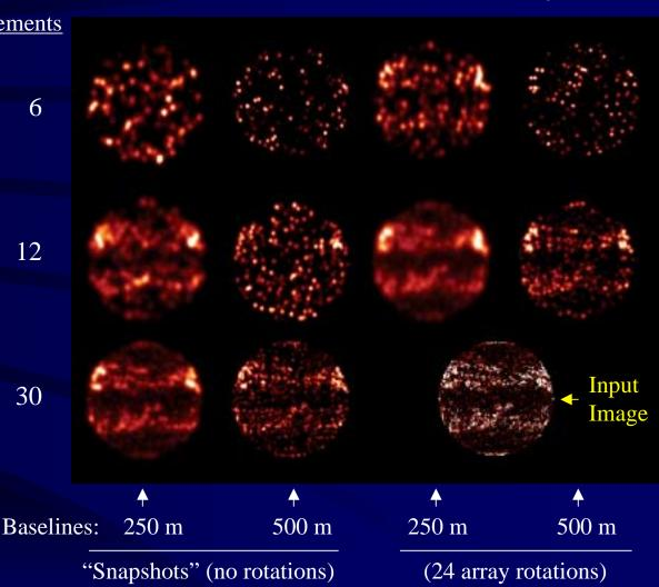
Conclusion: 30 static elements appear to be sufficient to adequately synthesize this stellar image, although 1 rotation of this array ought to improve things substantially still. Alternatively, fewer elements can be used with a larger number of rotations (6 elements/24 rotations or 12 e/6 r).
